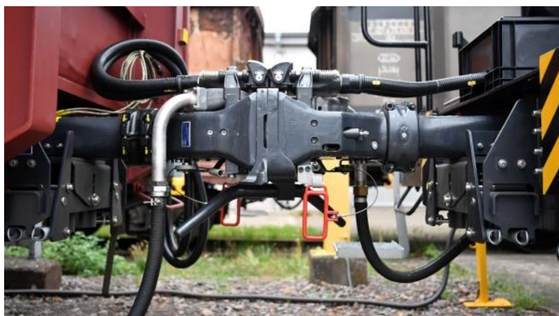
Figur 35 - Digital automatisk kobbel (International Railway Journal)
