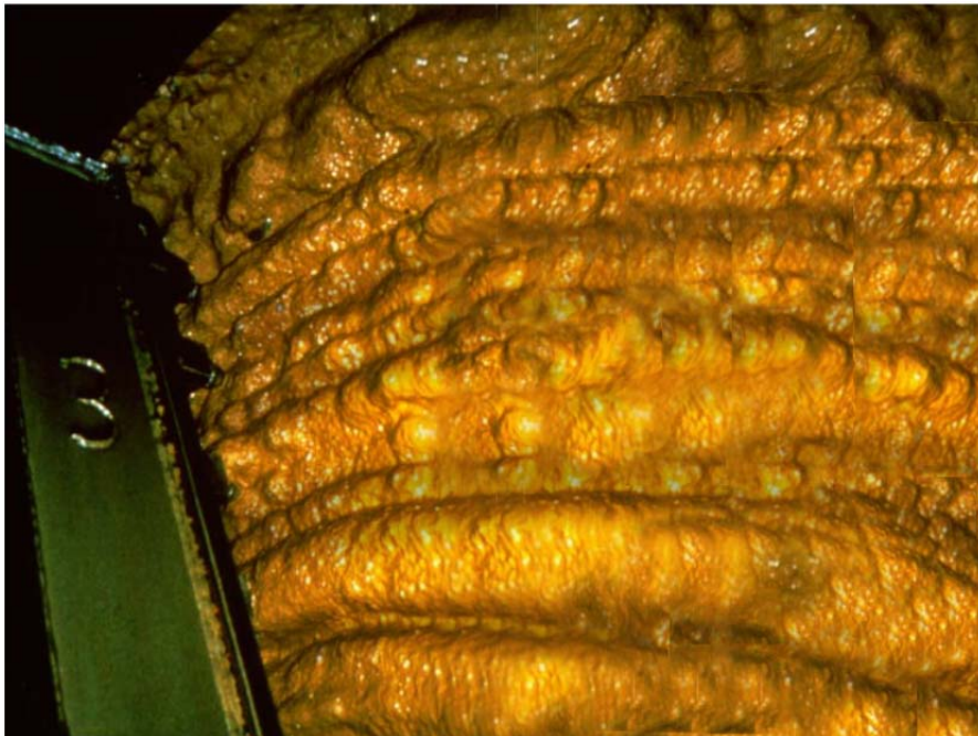
Figure 16: Impermeable filter cake
